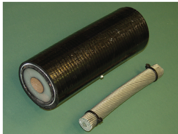
Underground cable and smaller overhead conductor.
